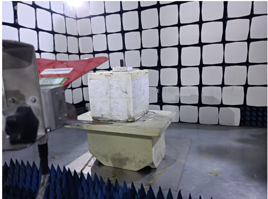
Radiation Emission Test Setup (1GHz to 18GHz)
