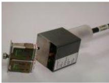
Serial optical link for communication with DASY4/5 embedded system (fully remote controlled) Two-step probe touch detector for mechanical surface detection and emergency robsot stop
