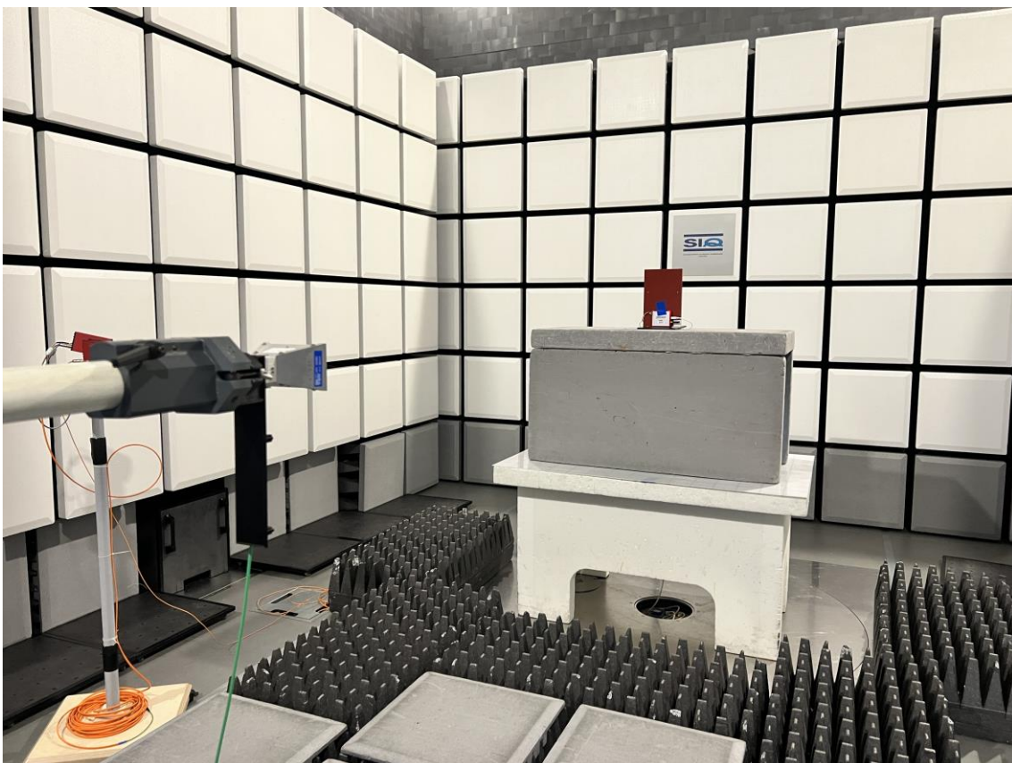
Figure 4: Spurious emission 18- 26 GHz
