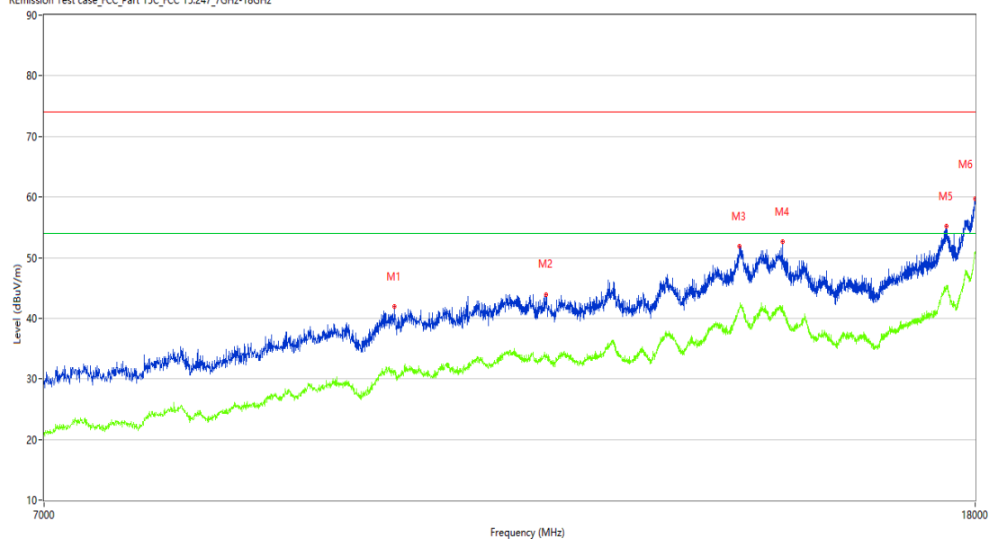
R Emission Test case_FCC_Part 15C_FCC 15.247_7GHz-18GHz
