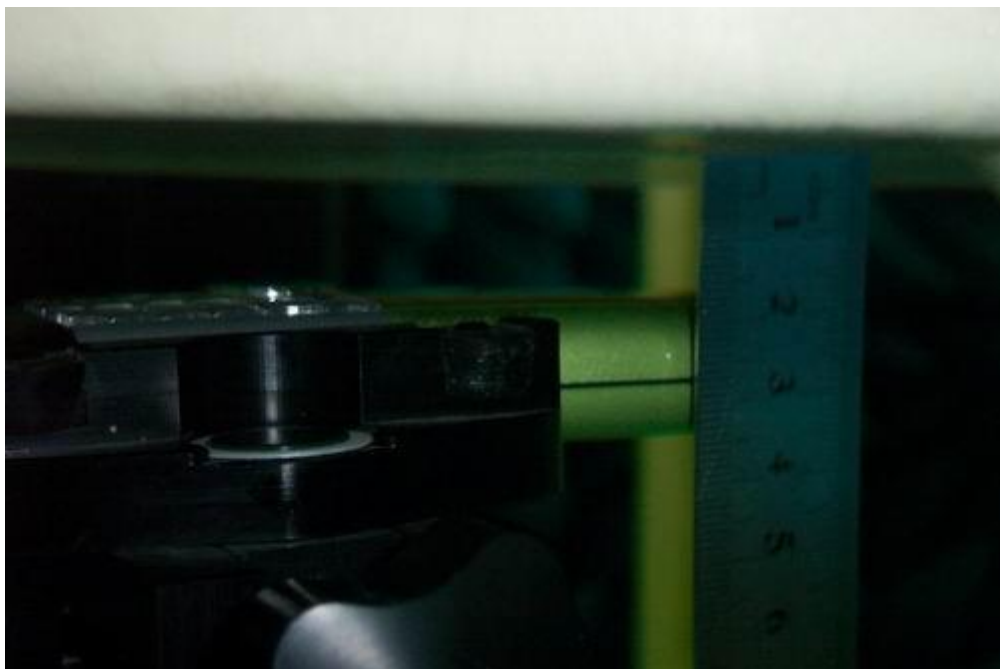
Picture 6 Flat Phantom -- Body-worn Position (toward phantom, the distance from handset to the bottom of the Phantom is 20mm)
