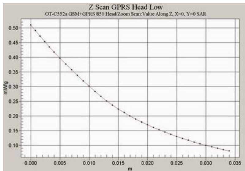
Fig. 98 Z-Scan at power reference point (Flat Phantom 850MHz GPRS CH128 with the display of the handset toward the phantom)
