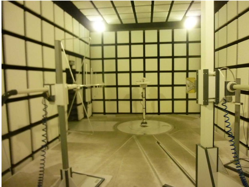
Photo 7: EUT at the anechoic chamber
