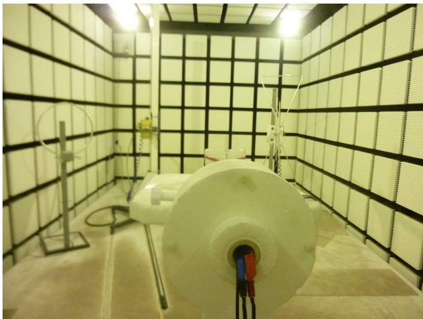
Photo 4: EUT at the anechoic chamber
