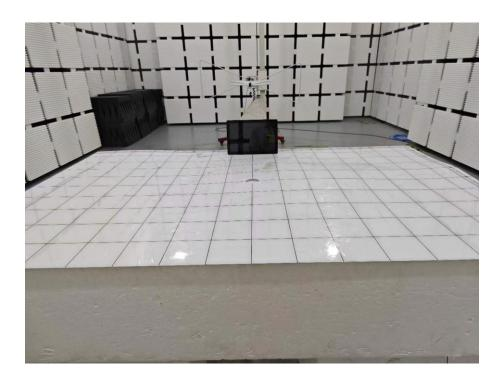
**Set-up for Radiated Spurious Emission, Above 1GHz**
