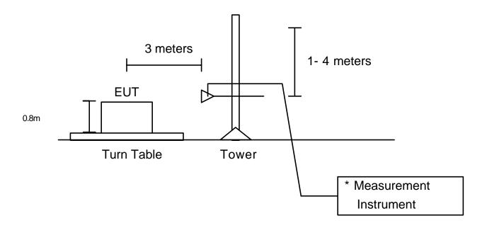
\* 30-1000 MHz, Rohde & Schwarz ESI40 receiver or 1-25 GHz, ESI40 with preamplifier and high-pass filter
