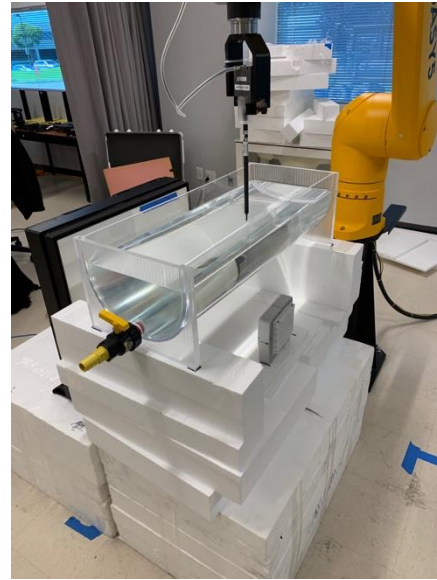
Figure 87: Half-cylinder phantom - partial obstruction
