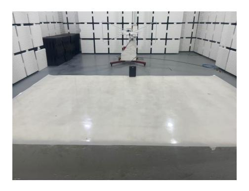
Set-up for Radiated Emission (RE), Above 1GHz
