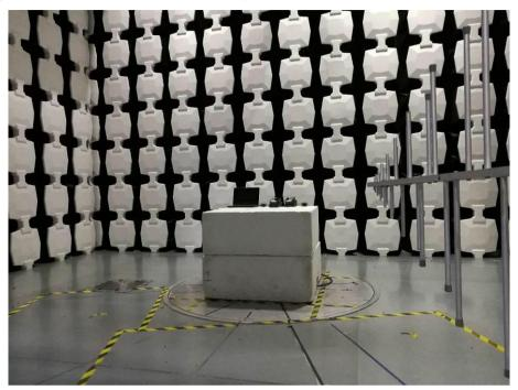
Description: Radiated Emission Test Setup
