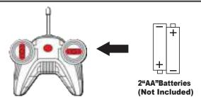
Use a screwdriver to open up the battery compartment located on the rear of your remote control.
