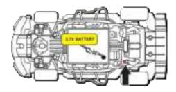
Move the power switch left and right to turn your car ON/OFF. Make sure to turn your RC car off when it is no longer used to preserve the battery charge.
