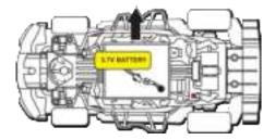
Open the drone's rear battery module and then pull the lithium battery out of the car battery compartment.
