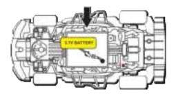
Once fully charged, insert the battery back into the battery compartment, making sure to connect it to the connector on the circuit board. Make sure when connecting not to reverse the positive and negative poles (+,-).
