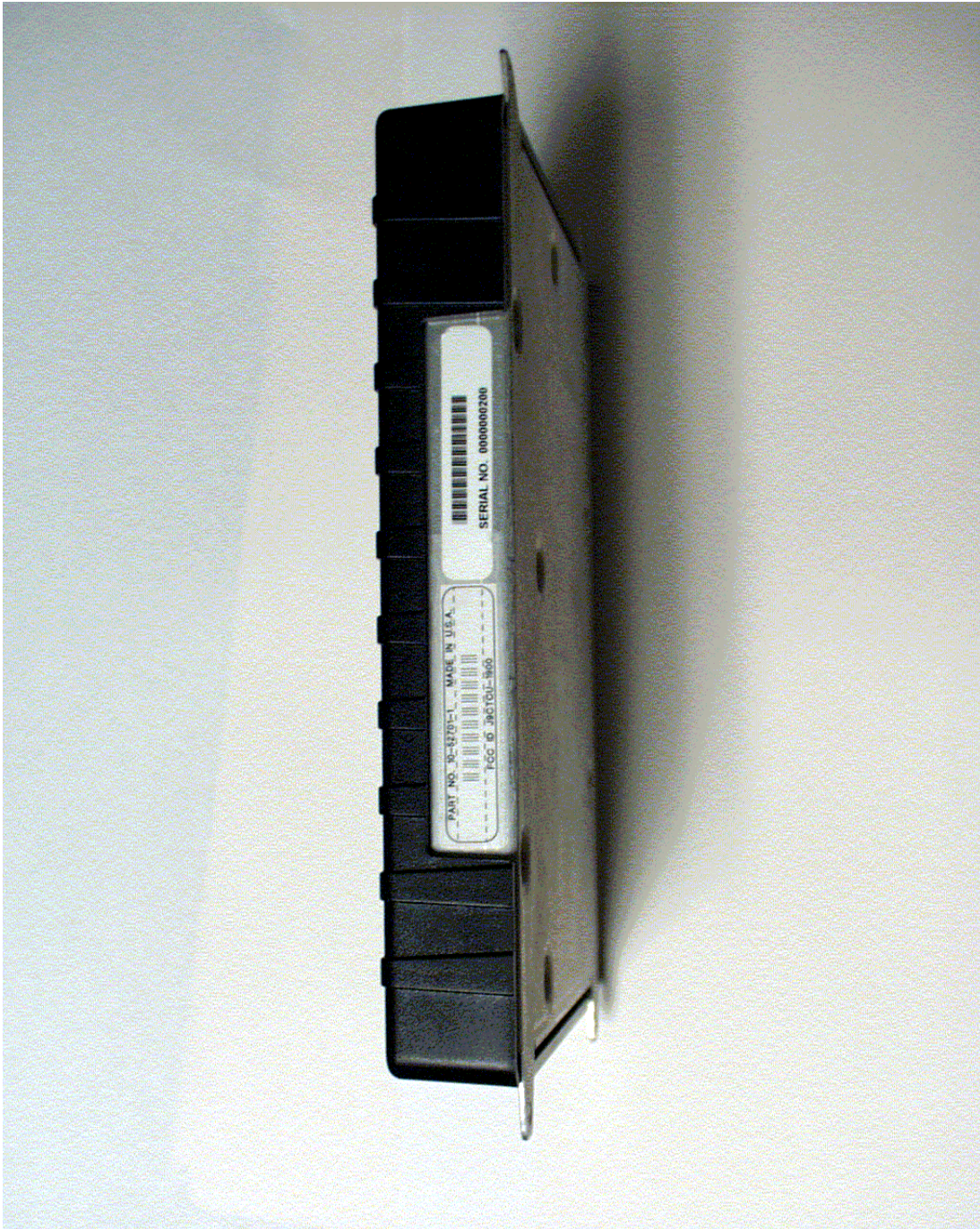
Figure 11–1. Label and its location for FCC ID J9CTCU-1900
