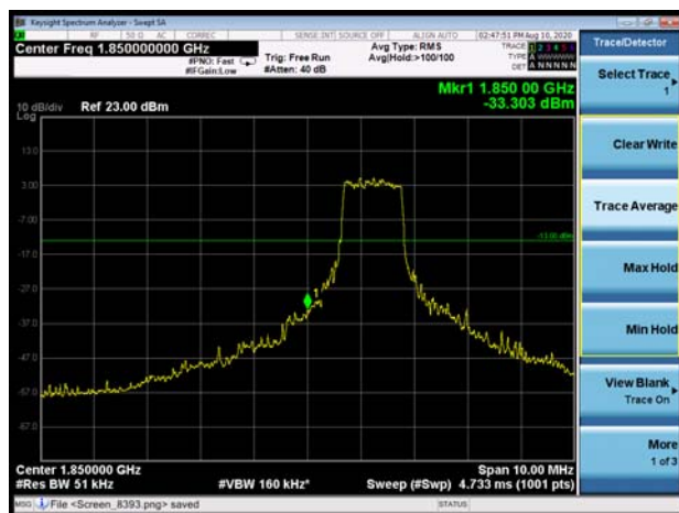
LTE Band 2 15MHz QPSK 1RB CH-Low
