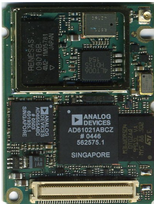
TC63: component side shielding opened
