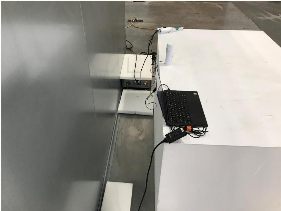
**Photograph 4: Back View Test Set Up Conducted Emissions**
