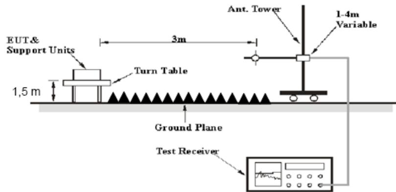
The radiated emission below 1GHz tests were performed in the 3 meters chamber test site A, above 1GHz tests were performed in the 3 meters chamber test site A, using the setup accordance with the ANSI C63.10-2013. The specification used was the FCC 15.209, and FCC 15.247 limits.
