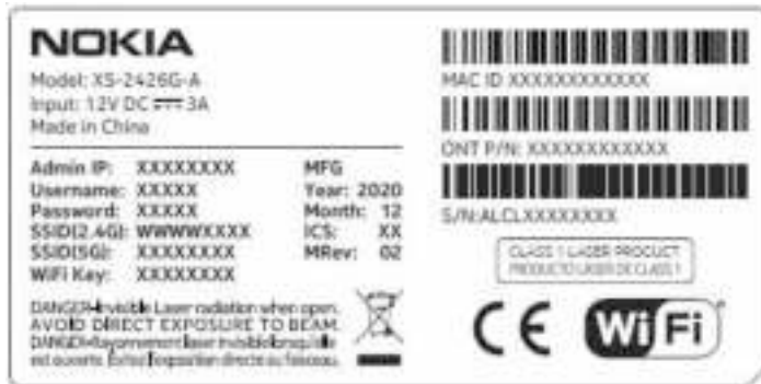
Figure 4-2 Sample laser product label showing CDRH 21 CFR compliance
