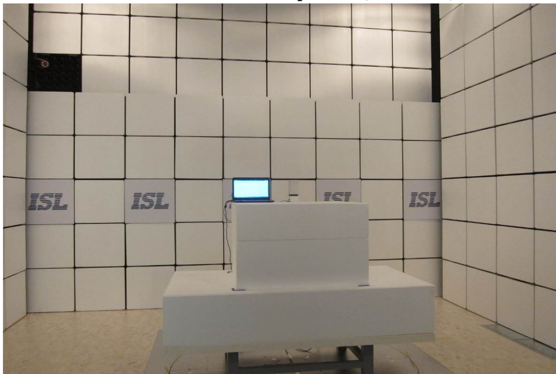
Radiated Emission Set up Photo (above 1GHz)
