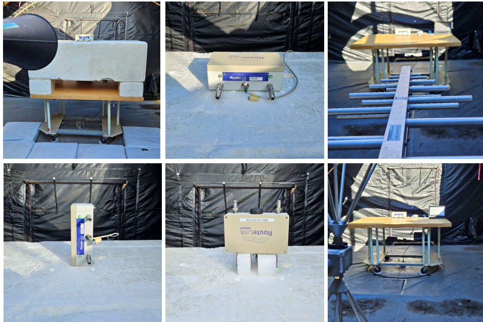
Figure 4.1.1 Radiated Emissions Test Setup Photograph(s).
