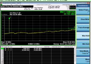
Test Mode: LTE Band 2 / 1.4MHz /6 RB
