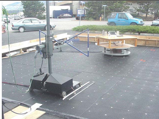
Photograph I.8-4 - 3115 Horn Antenna (2GHz - 10GHz)
