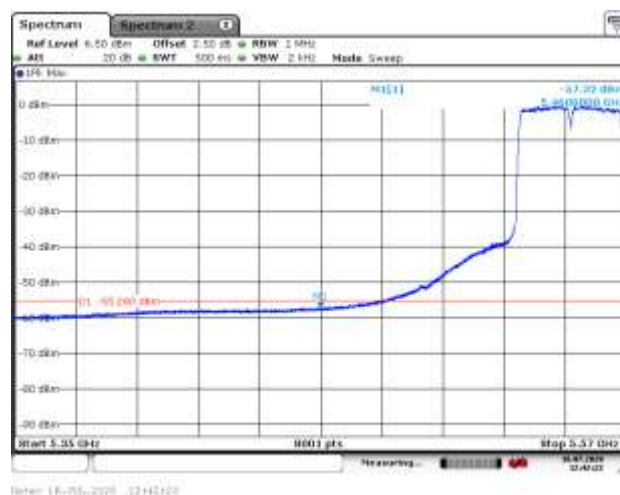
5795MHz with 2*2 Beamforming PK
