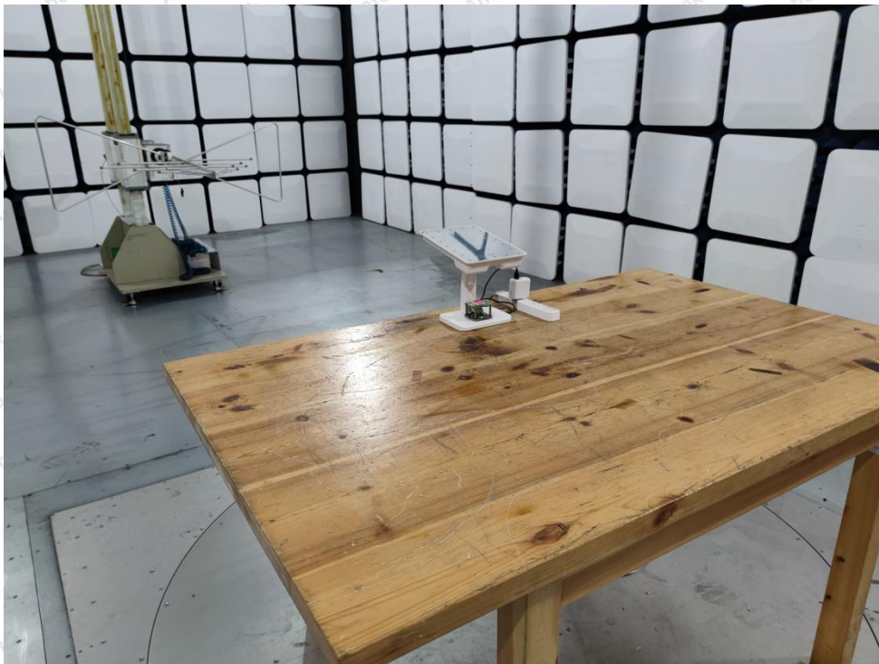
Photo of Radiation Emission Test
