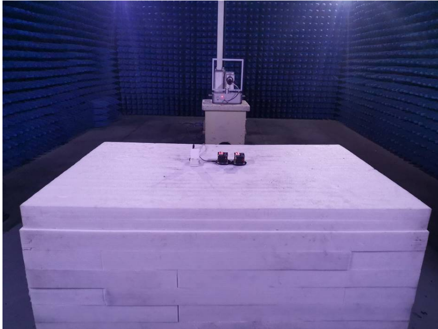
Photo of Radiated Emission Measurement (Below 1GHz)
