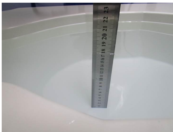
Liquid Height for Body SAR
