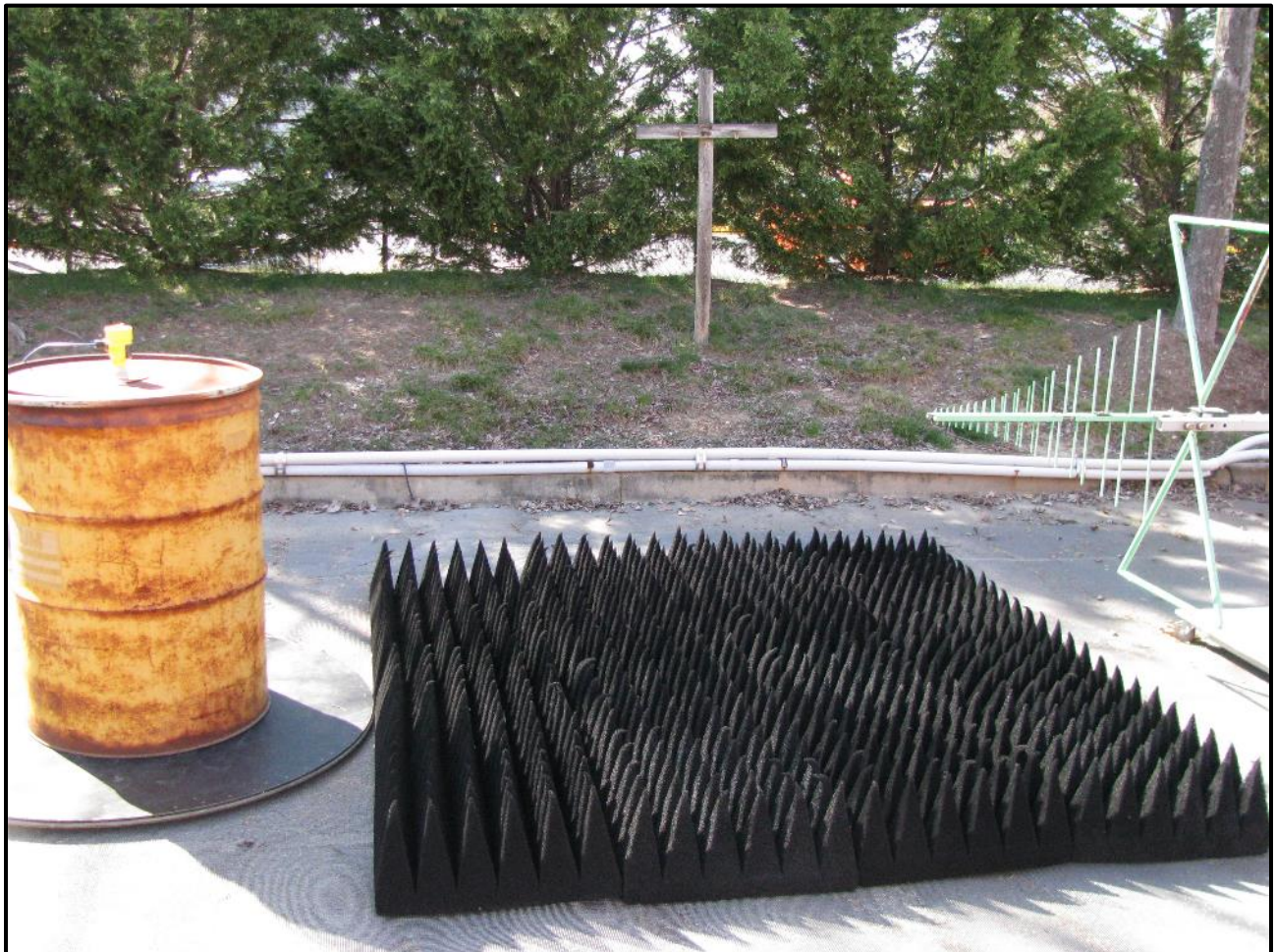
Photograph 23: Radiated Emissions – TC #6; Steel Container, Front View
