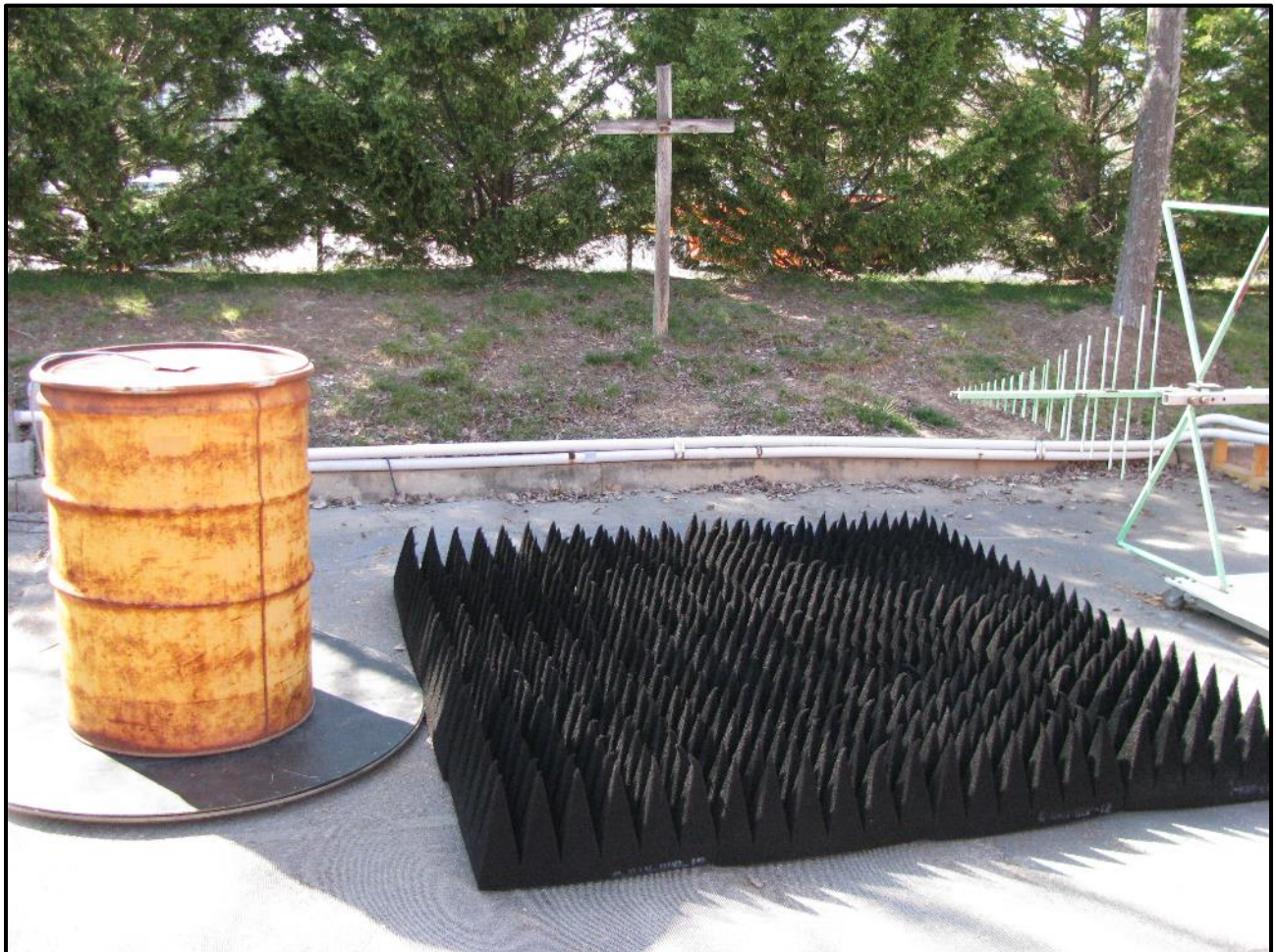
Photograph 27: Radiated Emissions – TC #8; Steel Container, Front View
