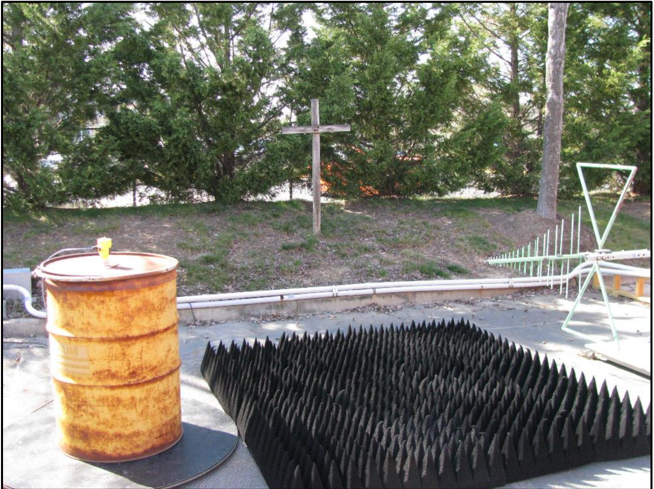
Photograph 15: Radiated Emissions – TC #2; Steel Container, Front View
