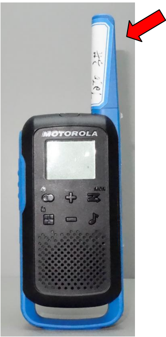
Fixed Antenna (front)
