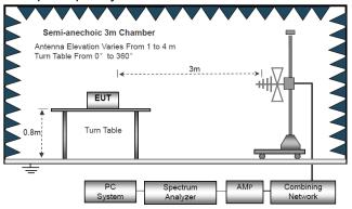
(C) Radiated Emission Test-Up Frequency Above 1GHz
