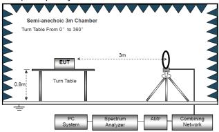
(B) Radiated Emission Test-Up Frequency 30MHz~1GHz
