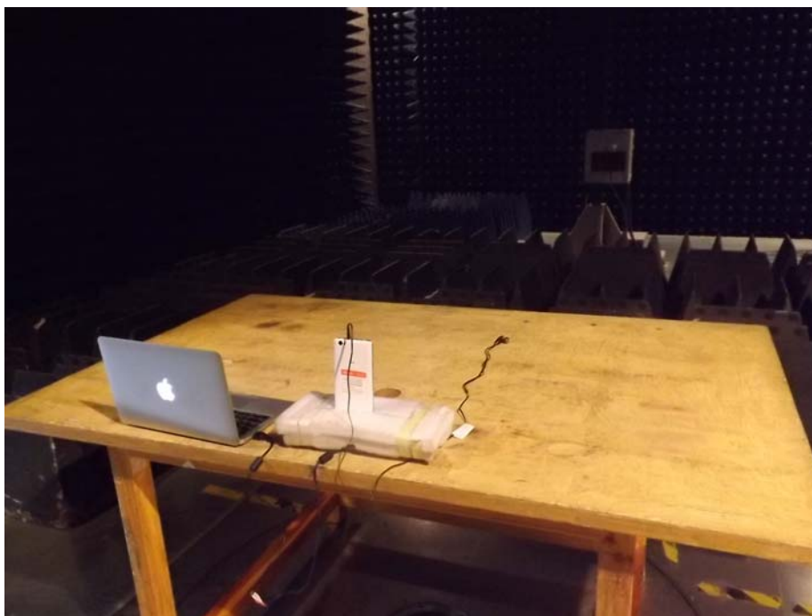
Photograph – Radiated Emission Test Setup for Above 1GHz at Test Site 1#
