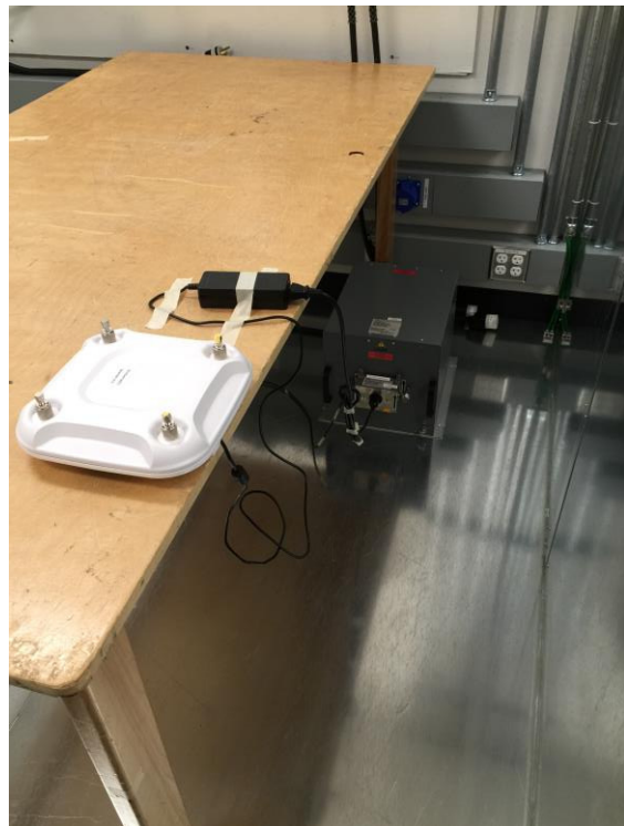
AIR-CAP3702P-B-K9 AC Conducted Emissions setup photo
