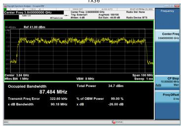
Test Model 3.1a Modulation 256QAM Channel Frequency 3934.98MHz
