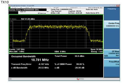
Test Model 1.1 Modulation QPSK Channel Frequency 3710.01 + 3890.01 MHz
