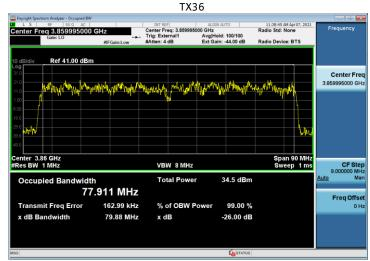
Test Model 3.1a Modulation 256QAM Channel Frequency 3920.01 + 3960 MHz
