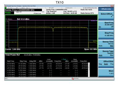
Test Model 3.2 Modulation QPSK/16QAM Channel Frequency 3840 + 3859.99 MHz
