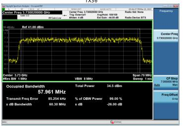
Test Model 3.2 Modulation QPSK/16QAM Channel Frequency 3840 MHz TX36
