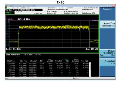
Test Model 3.2 Modulation QPSK/16QAM Channel Frequency 3840 MHz
