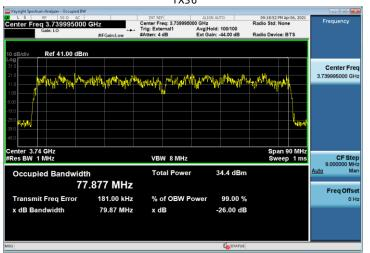
Test Model 3.2 Modulation QPSK/16QAM Channel Frequency 3840 + 3859.99 MHz
