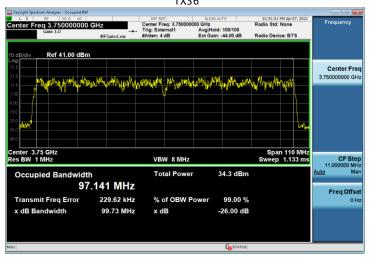
Test Model 3.2 Modulation QPSK/16QAM Channel Frequency 3840 + 3889.99 MHz TX36
