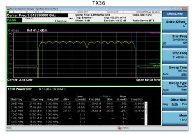
Test Model 3.1a Modulation 256QAM Channel Frequency 3950 + 3969.99 MHz
