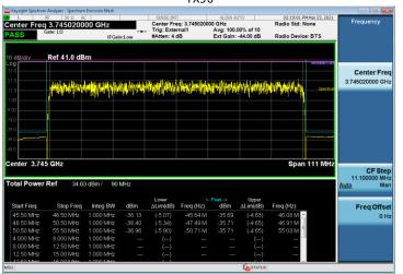
Test Model 3.1a Modulation 256QAM Channel Frequency 3934.98MHz
