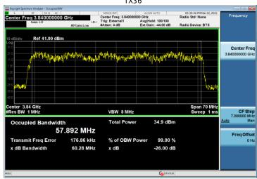
Test Model 3.1a Modulation 256QAM Channel Frequency 3949.98MHz
