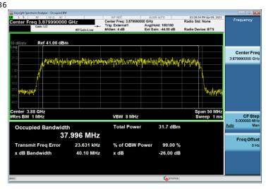
Test Model 3.1 Modulation 64QAM Channel Frequency 3800.01 + 3960 MHz
