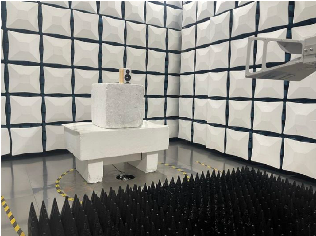
Photograph 3: Set-up for Radiated Spurious Emission, above 1GHz
