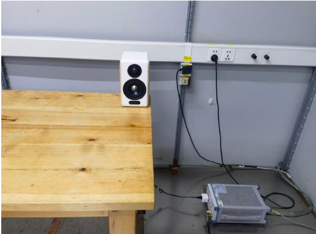
Photograph 1: Set-up for Conducted Emission on AC Mains
