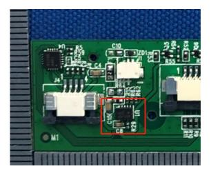
2. The new product delete AW IC (The AW IC only controls the brightness of the indicator LED)
