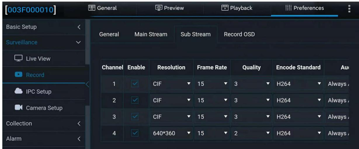
1. **Enable:** Sub-stream recording is enabled for a specific channel after this option is selected.
