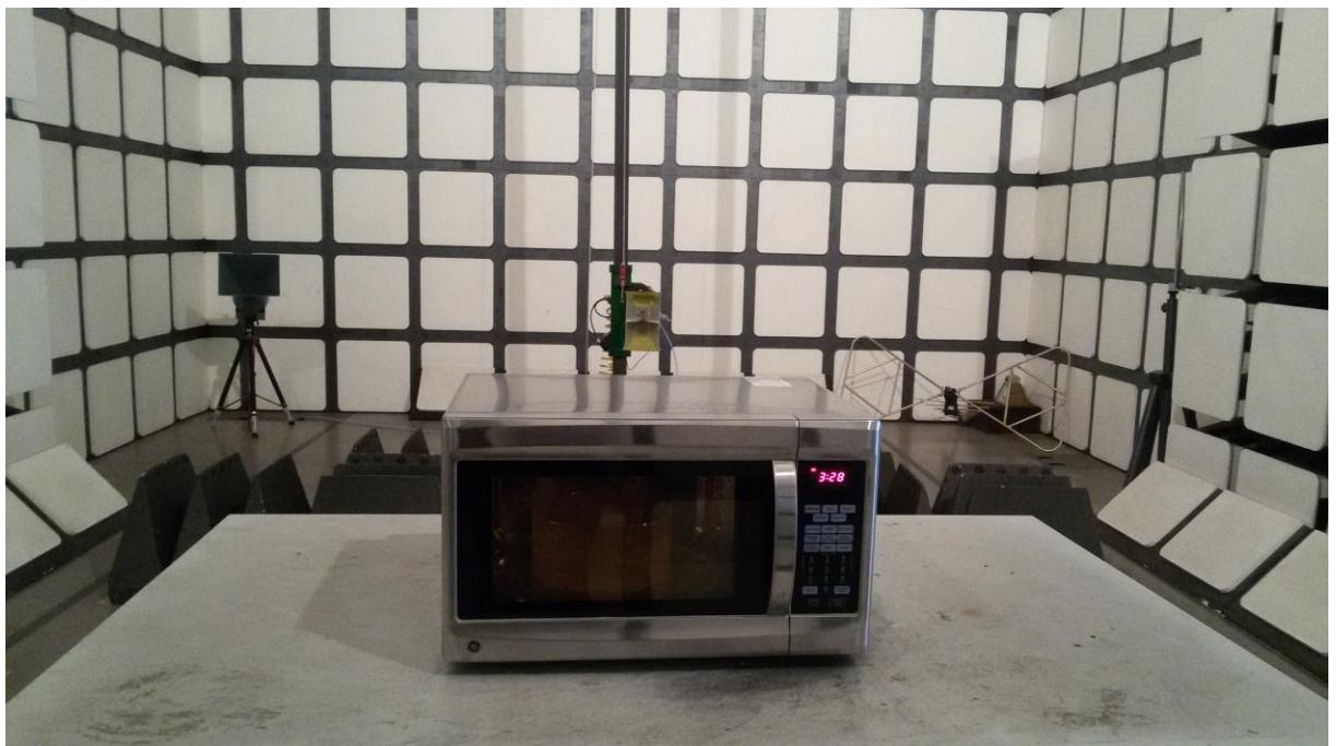
Radiated Emission Test Set-up (1-25GHz):
