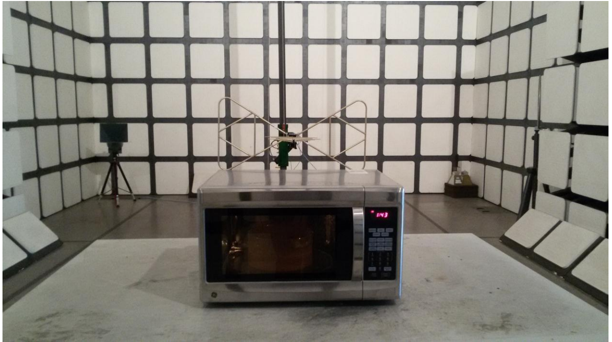
Radiated Emission Test Set-up (30 -1,000MHz):
