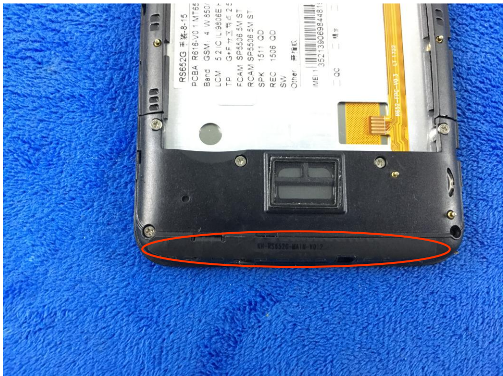
GSM/PCS/UMTS-FDD Antenna View
