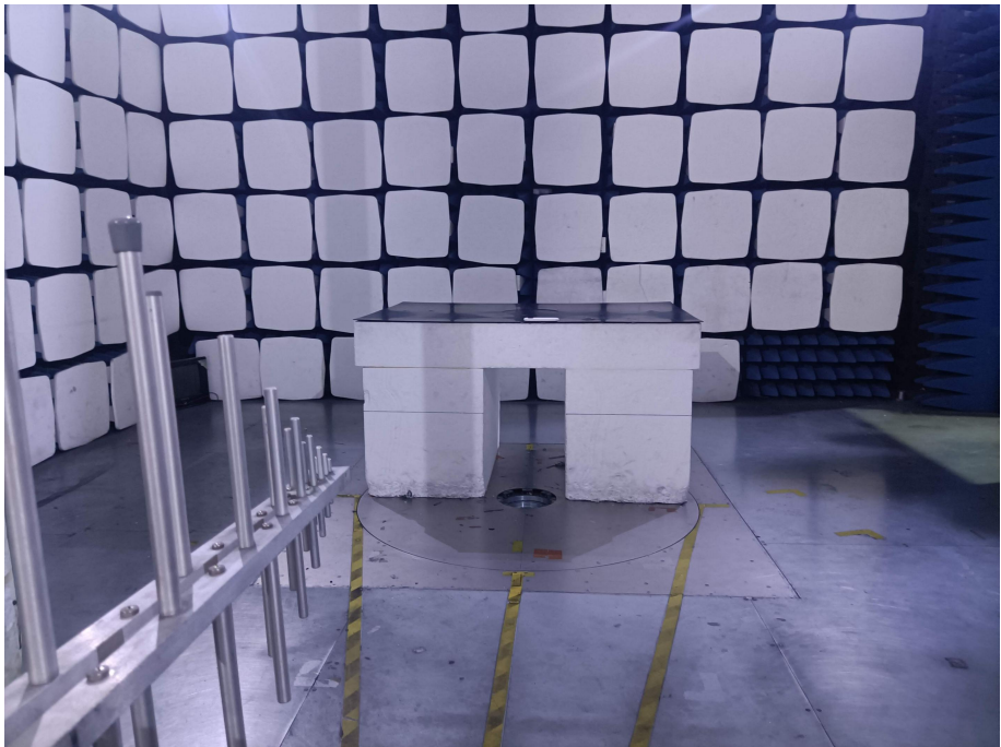
Radiation Emission Test Setup (30MHz to 1GHz)
