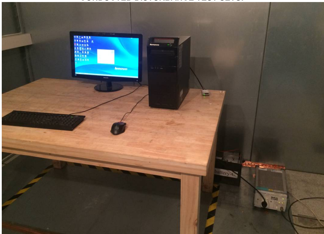
CONDUCTED DISTURBANCE TEST SETUP
