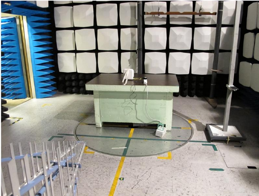
Test set up radiated emission 30 MHz – 1GHz
