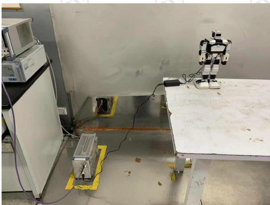
Conducted Emissions Test Setup
