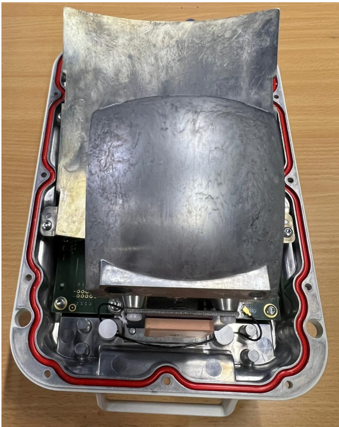
60 GHz cnWave V2000 Radome Removed Top View
