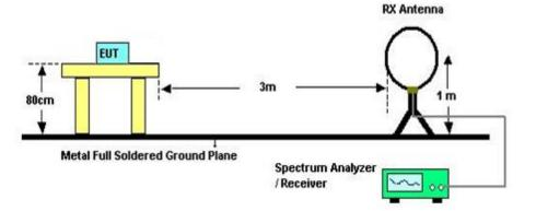
The setting of the spectrum Analyzer
