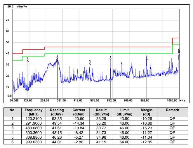
Note: 1. Result Level = Read Level + Antenna Factor + Cable loss.
