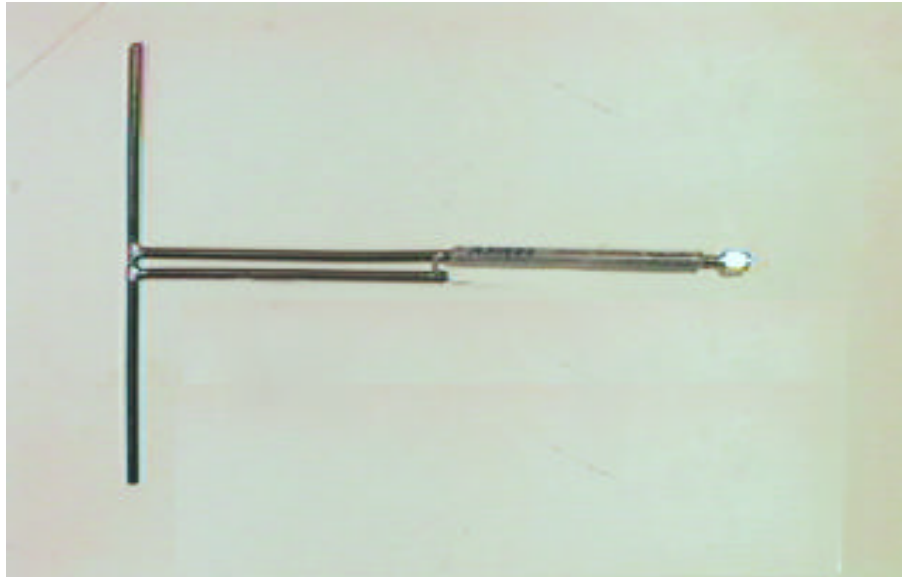
Reference Dipole Antenna Used for ERP Measurement
