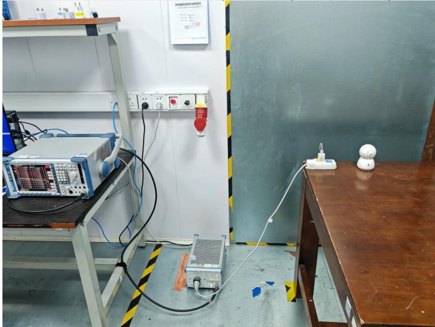
Conducted emissions at AC power line (150kHz-30MHz)
