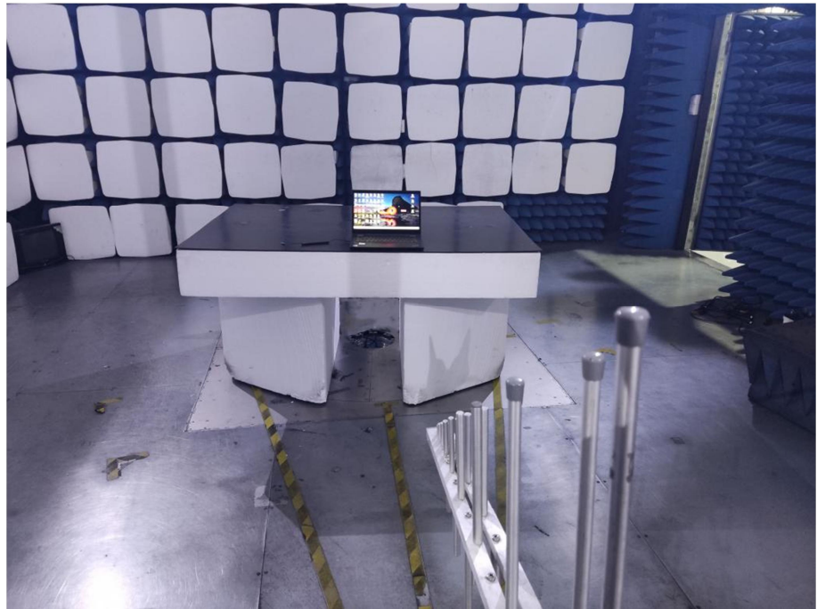
Radiation Emission Test Setup (30MHz to 1GHz)
