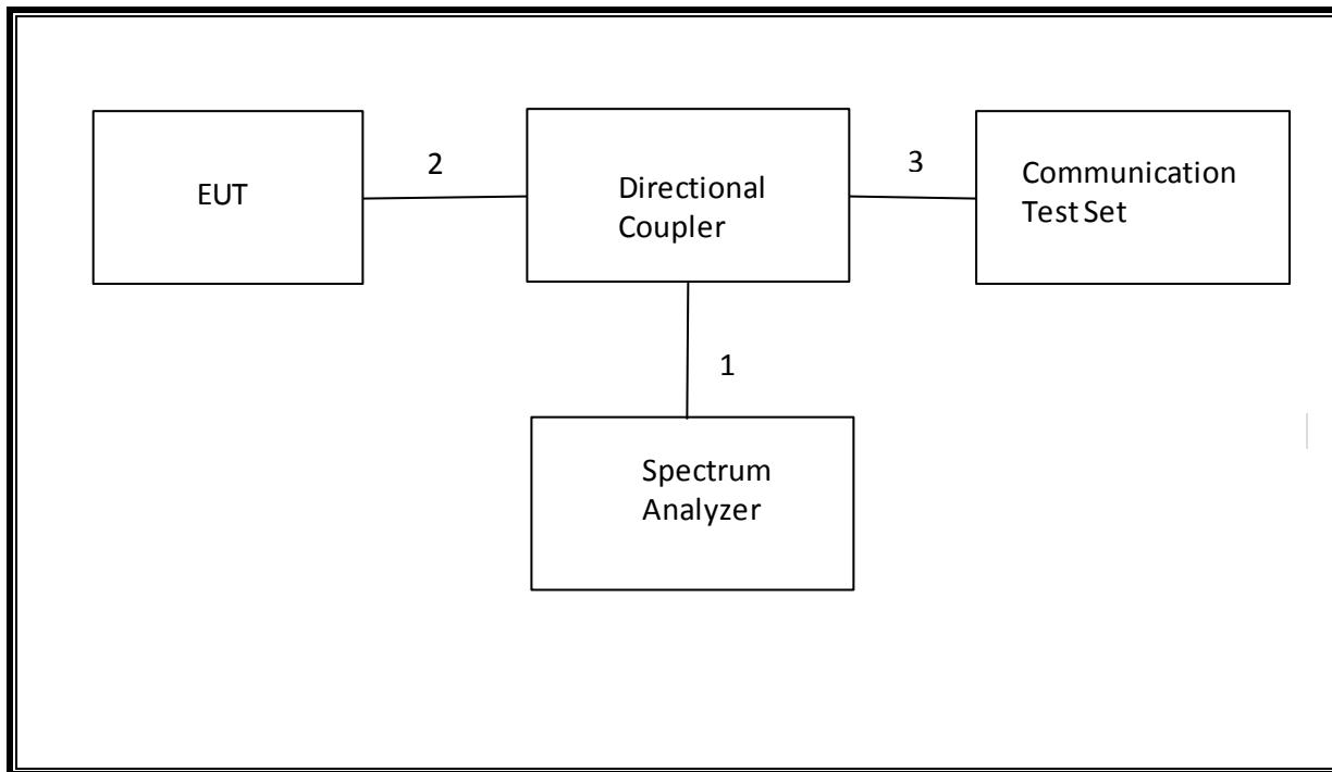
**SETUP DIAGRAM FOR TESTS (RADIATED TEST SETUP)**
