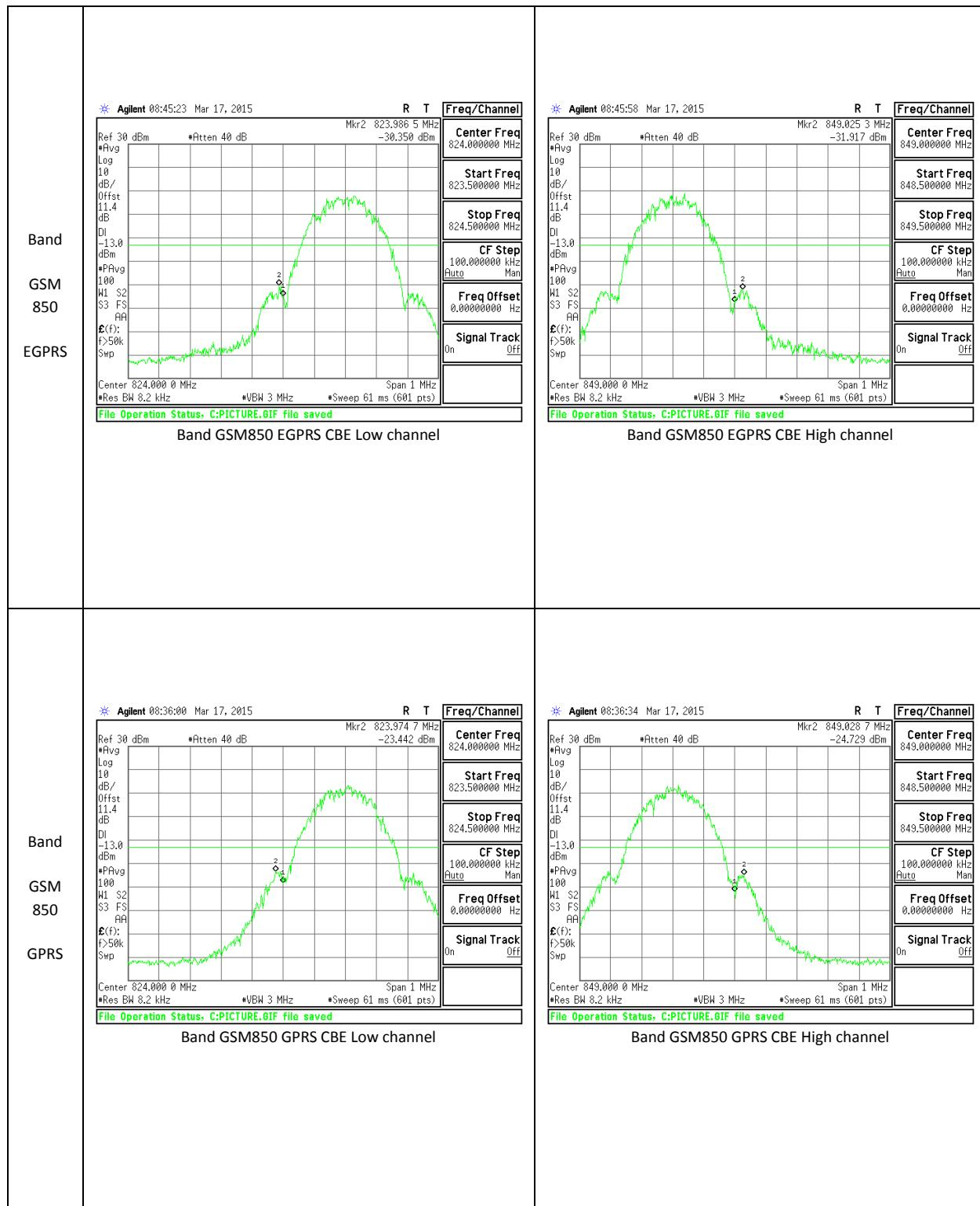
Note: GSM reading need add 9dB DCCF factor due to duty cycle is 12.5% during test.
