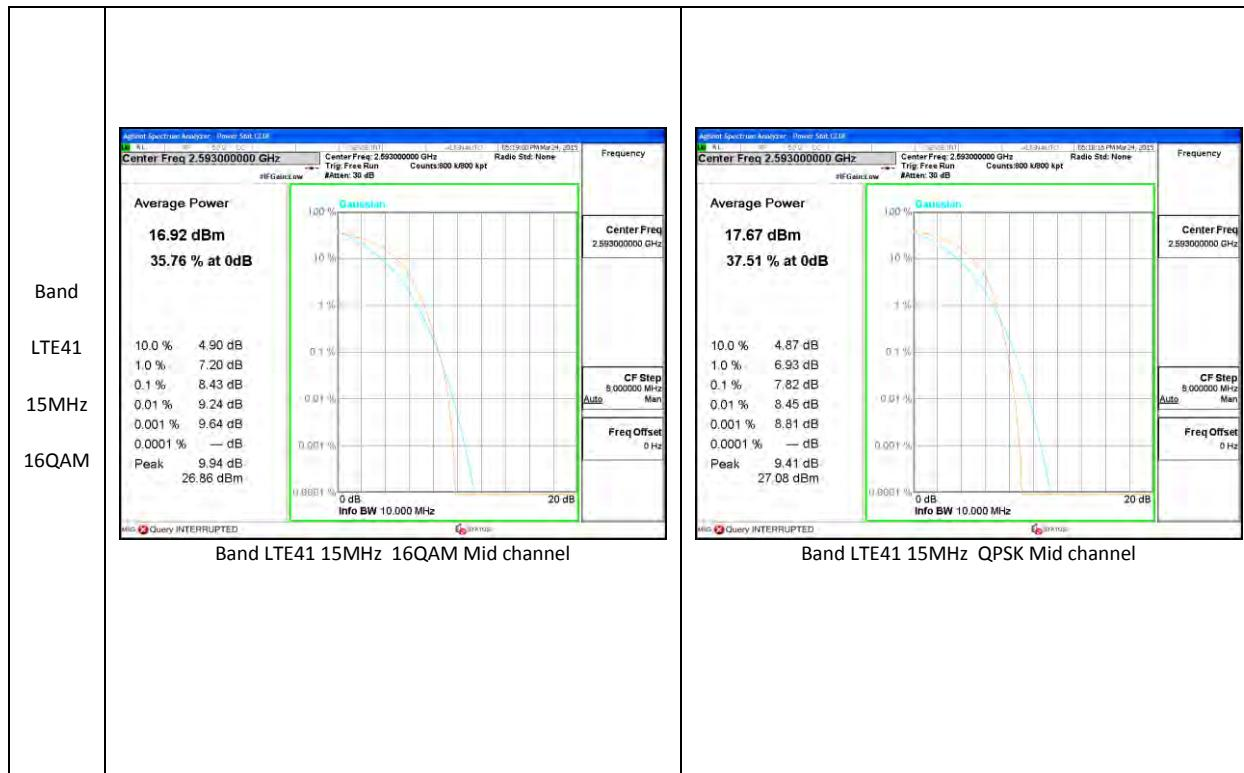
Band LTE41 15MHz 16QAM Mid channel
