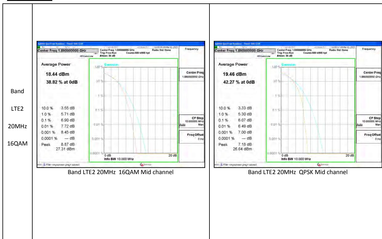
Band LTE2 20MHz 16QAM Mid channel
