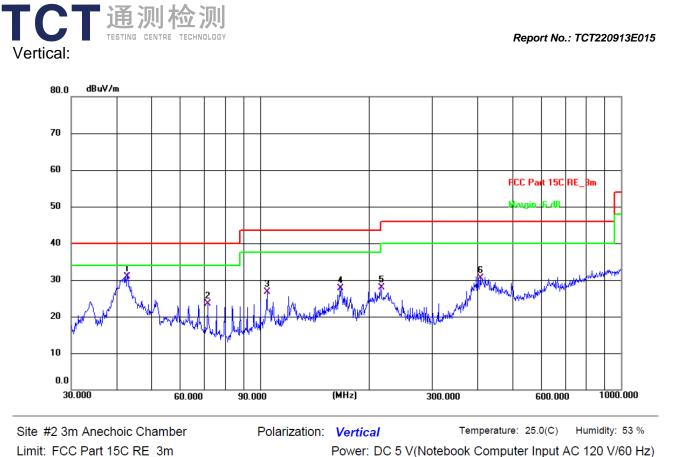
Margin Frequency Reading Factor Level Limit Detector P/F Remark No. (dB) (MHz) (dBuV) (dB/m) (dBuV/m) (dBuV/m) 42.8997 17.03 30.98 1 \* 13.95 40.00 -9.02 QP Ρ 2 71.5805 12.65 10.80 23.45 40.00 -16.55 QP Ρ 104.5360 15.94 10.77 26.71 43.50 -16.79 QP Ρ 3 166.6513 14.97 12.71 27.68 43.50 -15.82 QP Ρ 4 16.71 27.88 46.00 5 216.0239 11.17 -18.12 QP Ρ 407.5144 13.07 17.40 46.00 -15.53 6 30.47 QP Ρ
