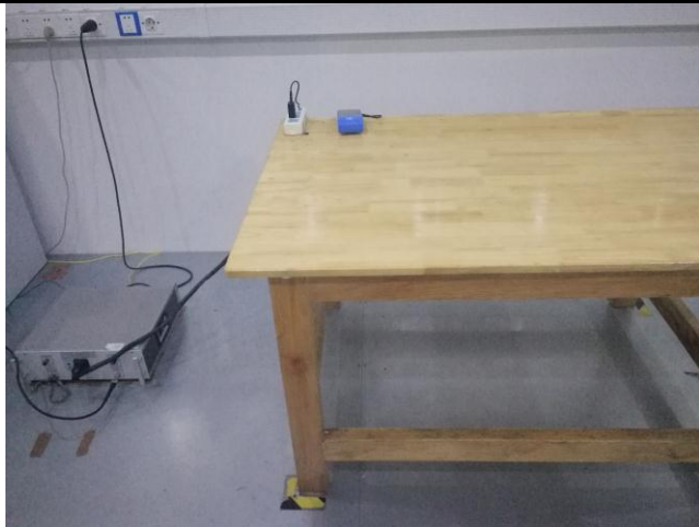
Conducted Emissions Test Setup Front View
