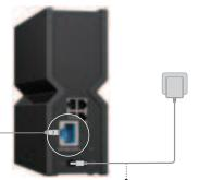
3 Connect the power adapter to the router.
